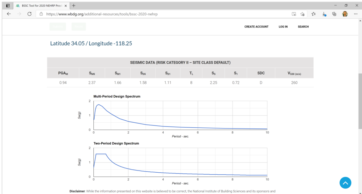
Figure 3-6. Example Output of the WBDG Web Interface to the USGS Seismic Design Web Service for the 2020 NEHRP Provisions and Thereby ASCE/SEI 7-22
